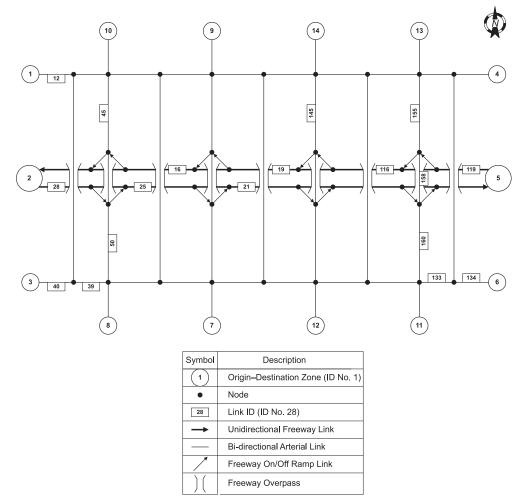
of a sample network used in the integration simulation model (M. Van Aerde 2000). The network represents a freewayarterial system consisting of 56 nodes and 124 links. An east–west freeway is located in the middle of the network surrounded by arterial links with a total length of 6.4 km.
